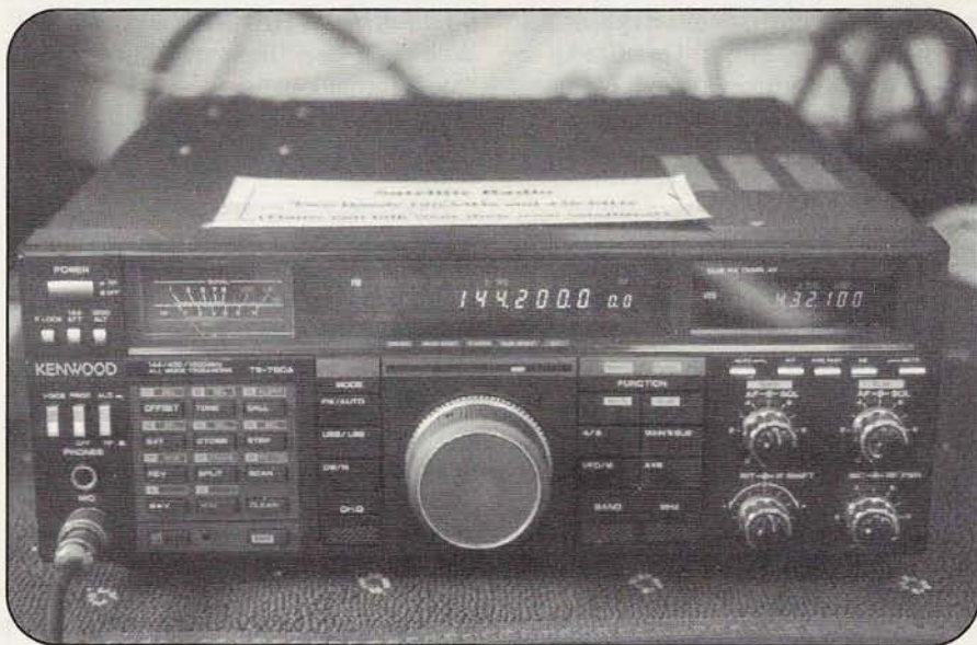
The massive (23-pound) Kenwood TS-790A on the test bench. No, it's not intended as a mobile rig even though it runs on 12 volts DC. It's built for home or portable operation where its excellent receiver can really be appreciated. (Photos by the author)
